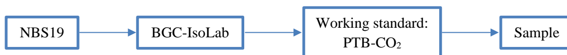
Figure 5 Example of a traceability chain for a set of experiments performed at PTB. These experiments aim at measuring the isotopic composition of CO 2 and interpreting it on a global scale. The internal working standards are measured at the BGL-IsoLab of the Max Planck Institute for Biogeochemistry in Jena, that provides traceability to NBS19, the scale-defining anchor for the VPDB scale.
