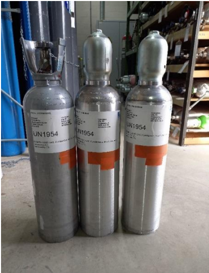
The 3 cylinders filled by Gasum with biomethane from their Lohja plant.
