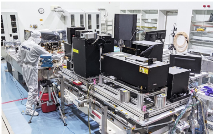
STAR-cc-OGSE pre-flight satellite calibration facility being used at Airbus Toulouse to characterise the CNES/UKSA MicroCarb instrument
