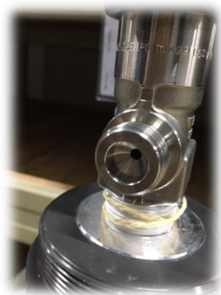
Figure 3 Typical stainless-steel cylinder valve
