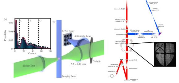
The left is the setup of our system, and the result of the Number-resolved imaging. The right is the plan for creating and imaging the tweezer array, and an image of 2-D array for the Durham University logo created with our SLM.
