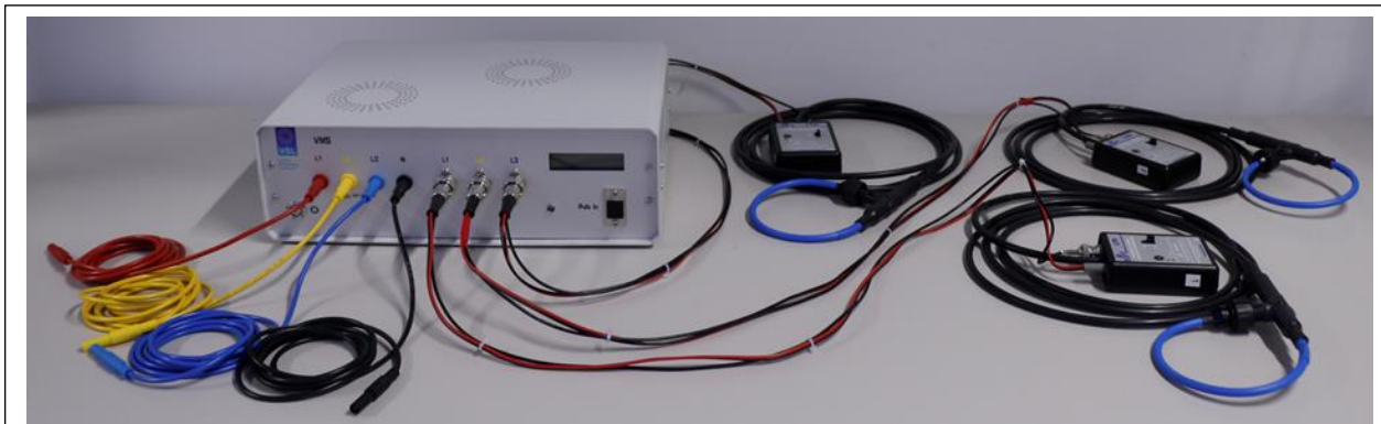
Fig.3 VSL 2-150kHz measurement system. Red, yellow and blue three pahse voltage input leads shown on left. Black boxes on right show Rogowski coils for 120 A or 1200 A peak current input in range 0.3 Hz - 150 kHz.
