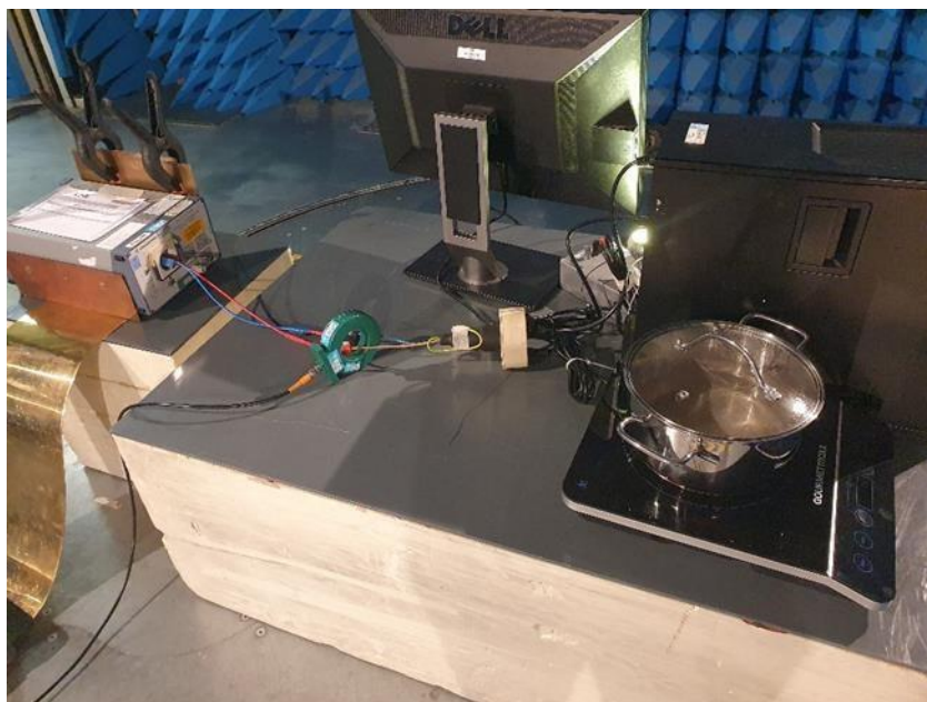
Fig.6, LNE Setup to measure harmonic emission for combined appliances: induction cooker, desktop computer and LED lamp
