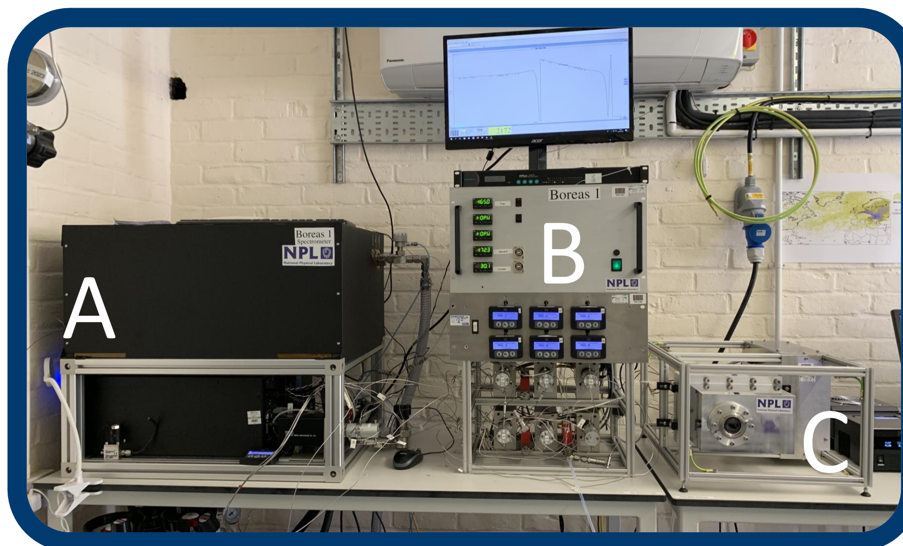
Figure 1: The Boreas methane (CH 4 ) preconcentration system (B-C) is coupled to a dual-laser spectrometer (A) for making simultaneous measurements of \delta^{13}\text{C}(\text{CH}_4) and \delta^2\text{H}(\text{CH}_4) in ambient air.
