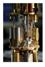
Metallic magnetic calorimeters (MMC) are particle detectors, typically operated at temperatures between 10 and 30 mK, that make use of paramagnetic sensors in conjunction with SQUID (Superconducting Quantum Interference Device) magnetometers to transform the temperature rise upon the absorption of radiation into a precise energy measurement. These devices achieve very high energy resolution and low energy thresholds.
