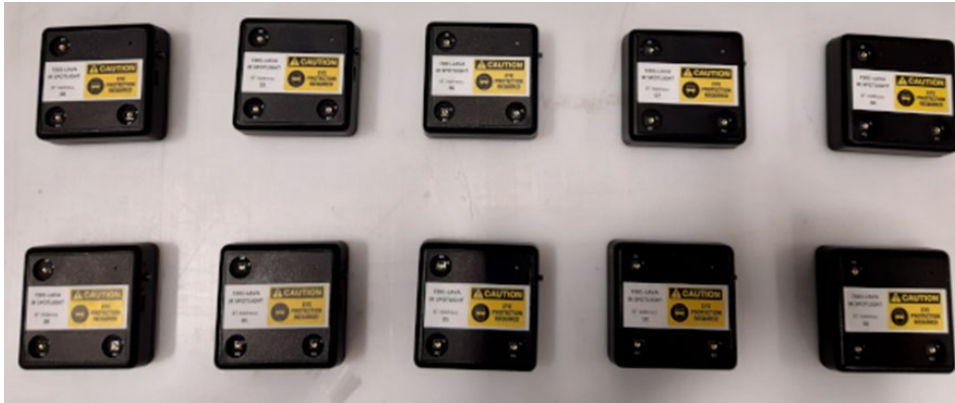
Figure 11 - self-powered active targets developed by TEKNIKER.
