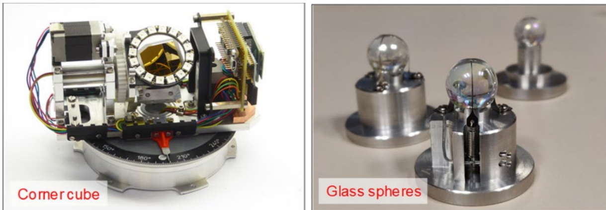
Figure 4 - the two type of reflector used in the CNAM system: left - hollow corner cube in motorised stage; right - glass spheres.
