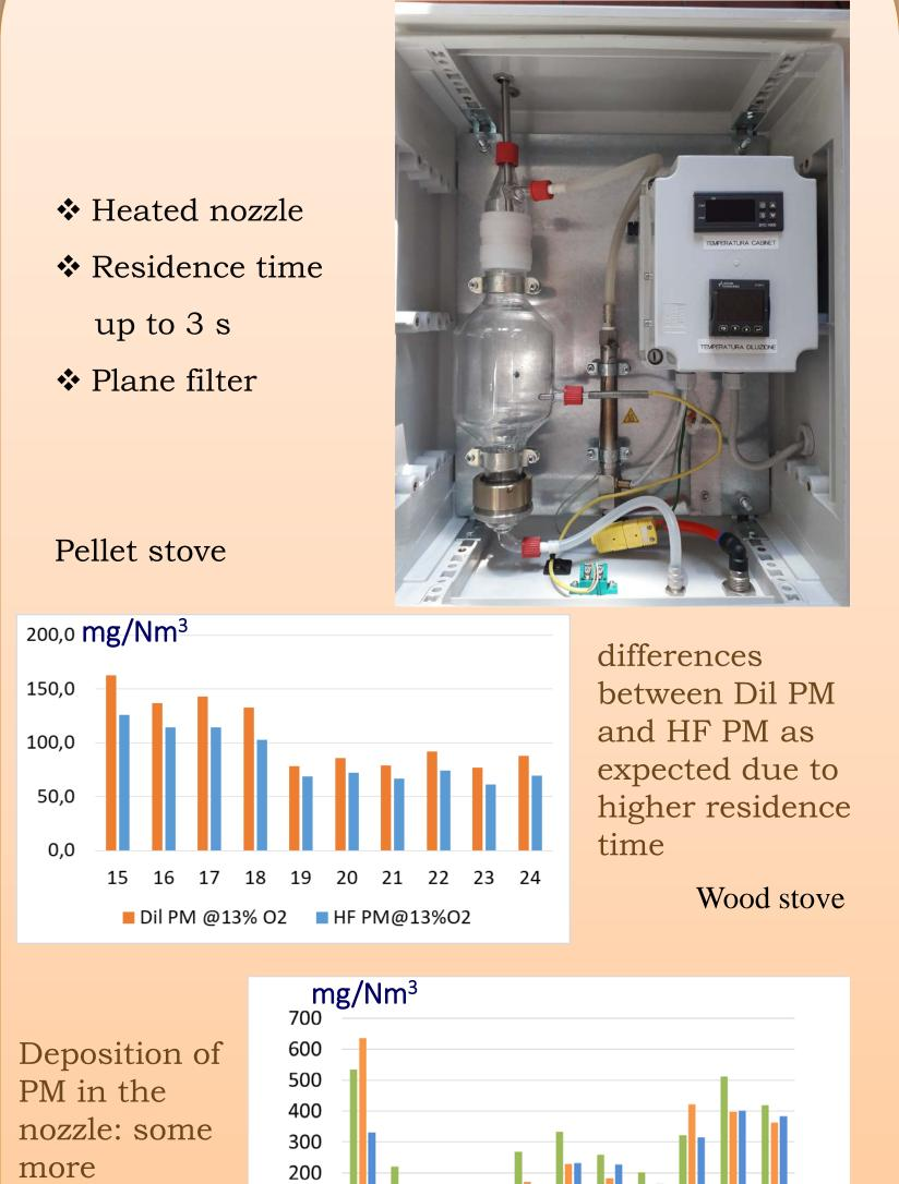
Dil PM appears lower than HF PM: loss of material
