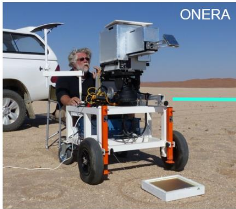
Figure 5: Mobile emissivity measurements of Gobabeb by ONERA
