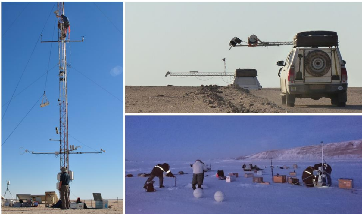
Figure 4: Examples of land and Ice surface temperature validation methods: tower at Gobabeb, FRM4STS comparison campaign in Gobabeb and buoys for ice temperature in Greenland.
