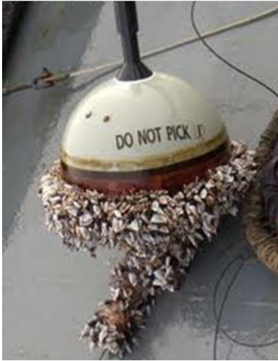
Figure 7: Taken from presentation of Minnett, showing state of ocean Buoy after a year at sea!
