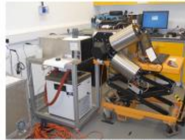
MAERI (UofM) viewing NPL ammonia Heat pipe
