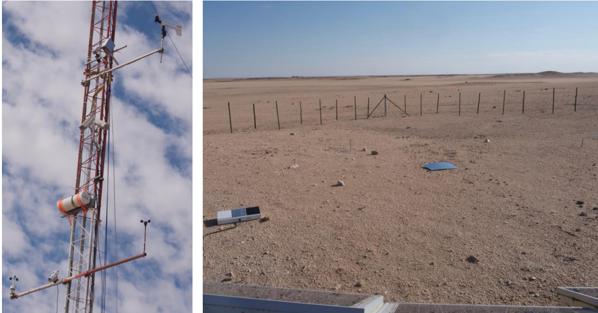
Figure 16 Left: radiometers at GBB Wind mast; the ISAR (white cylinder) is at 12m height. Right: the FOVs of the radiometers were aligned to the spot marked by the aluminium reflector (centre-right; removed for measurements).
