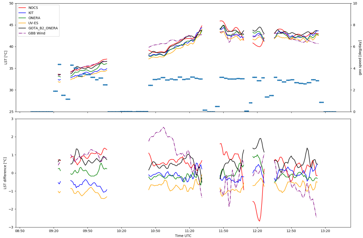
Figure 20 Top: in-situ LST retrieved on the 23 rd of June 2017 while driving across the gravel plains. The blue points refer to the right axis and give an estimate of vehicle speed: only in-situ LST for speeds > 2 deg/day (about 9.3 km/h) are taken into account. Bottom: differences between in-situ LST and mean in-situ LST determined. GBB Wind in-situ LST is shown for reference only (i.e. not included in mean LST).
