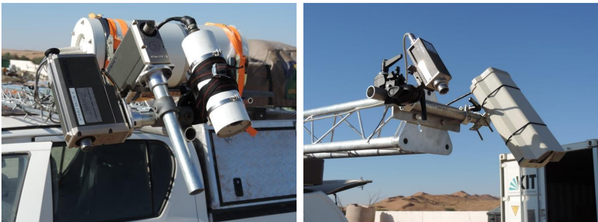
Figure 19 Close-ups of the radiometers mounted to the 4x4 vehicles. Left: ISAR (NOCS), KT19.85 II (ONERA) and CIMEL 312-2 (GOTA). Right: KT15.85 IIP (KIT) and CIMEL 312-1 (TRSG-UV).
