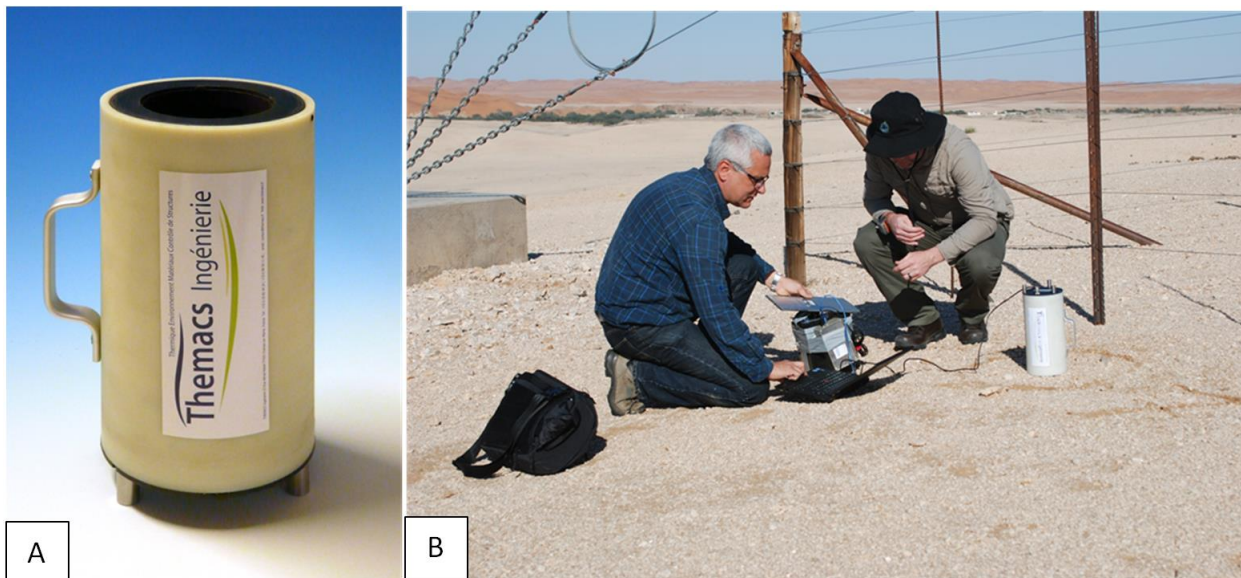
Figure 4. A: the sensor head of the EM3 emissiometer. B: field measurement on Gobabeb site
