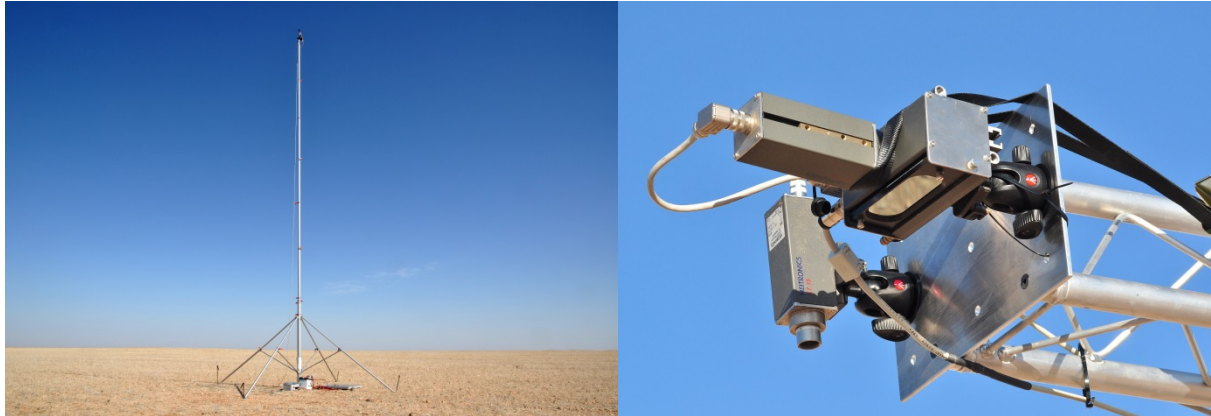
Figure 3: Telescopic mast on the gravel plains (left) and two radiometers and a scanner mounted to the horizontal beam on top of a 4x4 off-road vehicle (see Figure 4).
