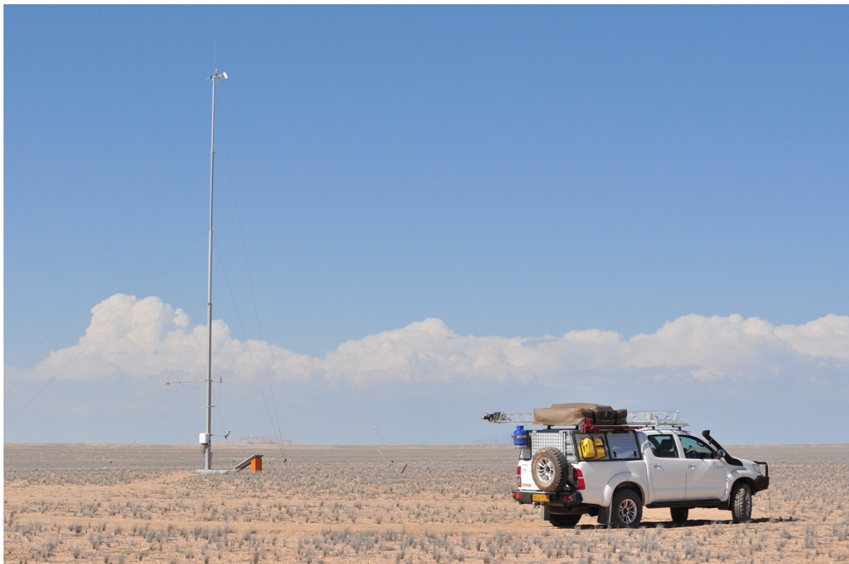
Figure 4: 'Station Plains' (see Figure 2) and 4x4 off-road vehicle with horizontal beam attached to its roof for performing mobile radiometric measurements across the gravel plains.
