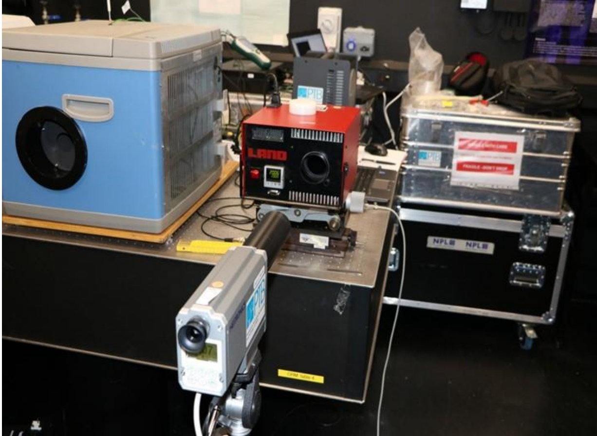
The KIT blackbody being measured by the PTB radiometer
