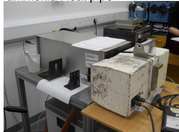
SISTER (RAL) viewing NPL ammonia Heat pipe
