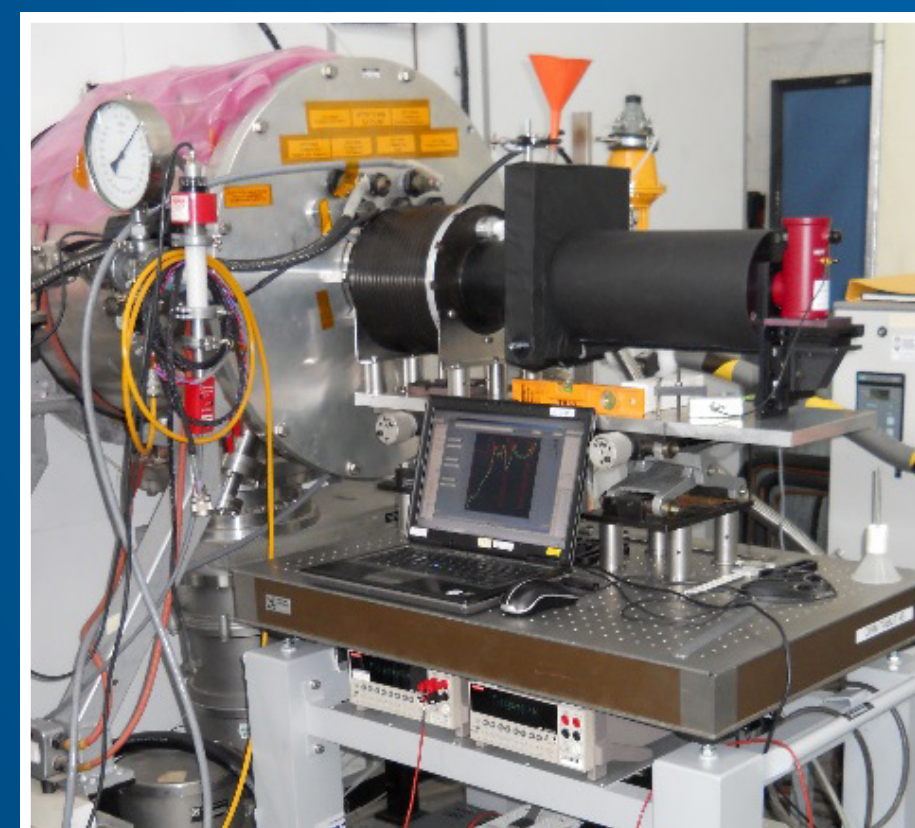
Figure 2: AMBER shown during the calibration of a space blackbody which is operating in the vacuum chamber.
