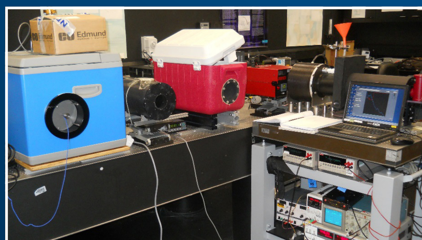
Figure 3: AMBER measuring the radiance temperature of a number of blackbodies during the 2016 FRM4STS blackbody comparison
