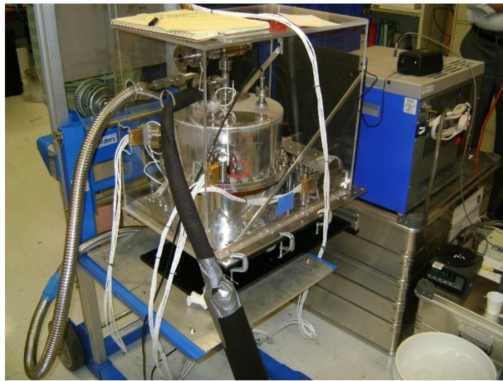
Figure 3: The NIST TXR radiometer monitoring the temperature of the Southampton University blackbody during the 2009 Workshop.
