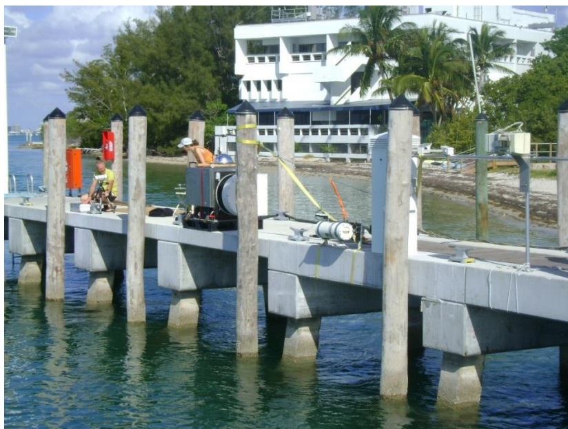
Figure 5: Participants' radiometers measuring the SST from the pier at Miami University during the 2009 Workshop. From the left to right, the radiometers of the University of Laguna, MAERI, ISAR and SISTER radiometer can be seen.
