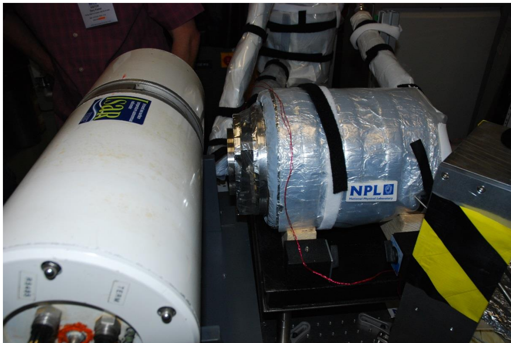
Figure 2: ISAR radiometer (on the left) monitoring the temperature of the NPL reference blackbody during the 2009 Workshop.
