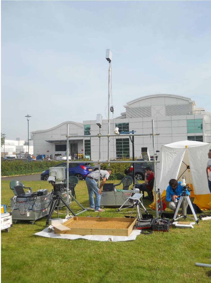
Figure 1: Radiometers mounted on the steel frame during the comparison of the surface temperature of the sand sample contained in the wooden frame.
