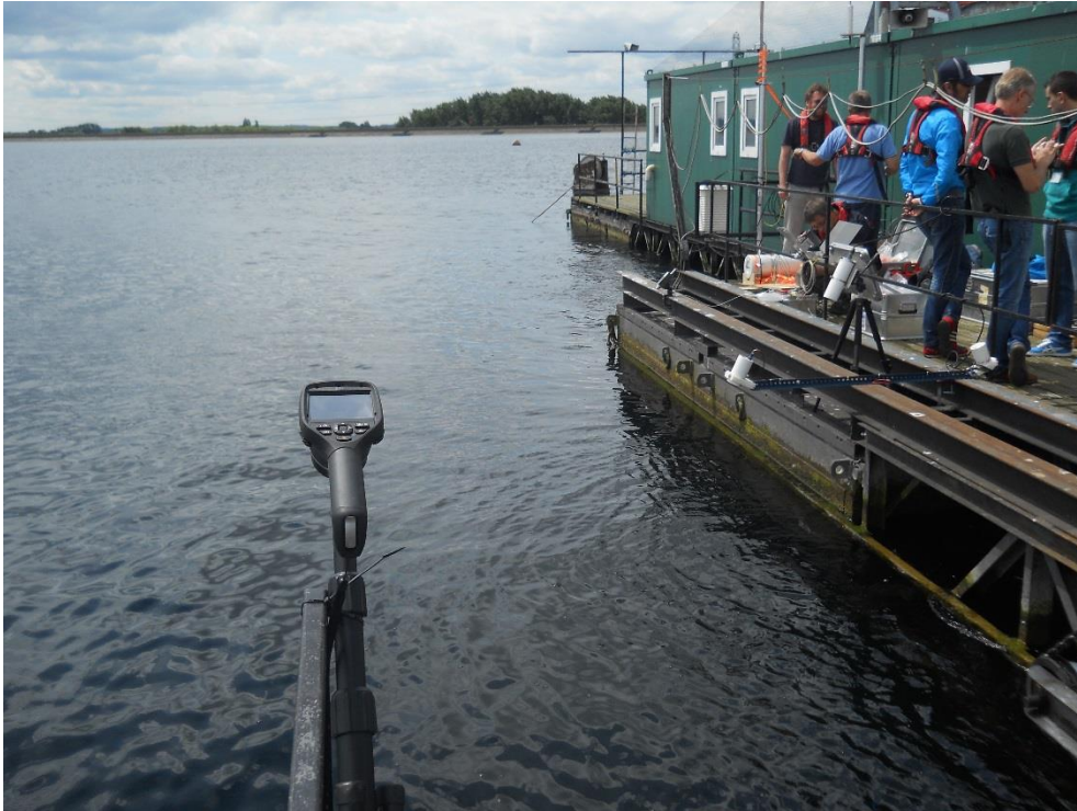
Figure 3.4: The thermal imager viewing the surface of the water. Note the ripples on the surface of the water which give rise to the temperature fluctuation which were observed in the thermal images recorded.
