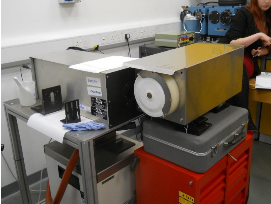
The OUCFIRST radiometer viewing the NPL reference blackbody
