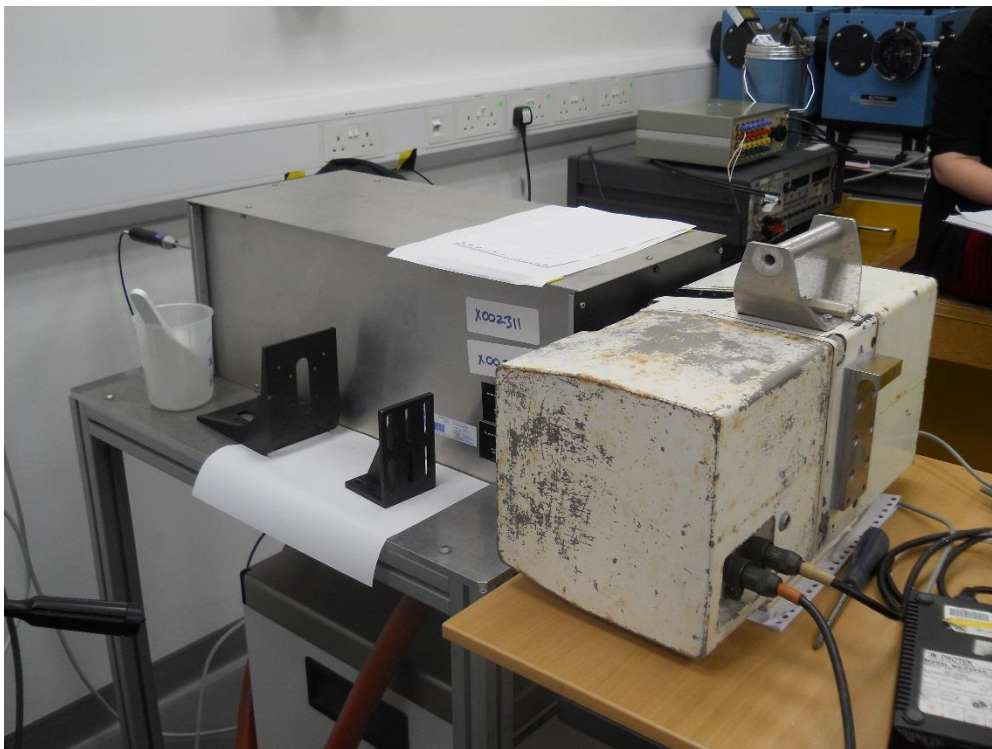
The STFC RAL SISTeR radiometer viewing the NPL reference blackbody.
