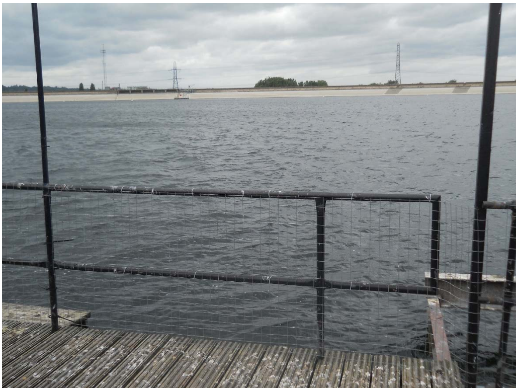
Figure 3: Another view of the platform showing the railings and the mesh which can be removed so the radiometers can be attached to the railings.
