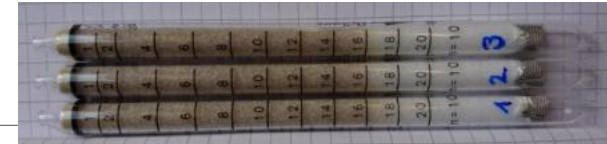
H 2 S measurement with Dräger; compressed raw biogas
