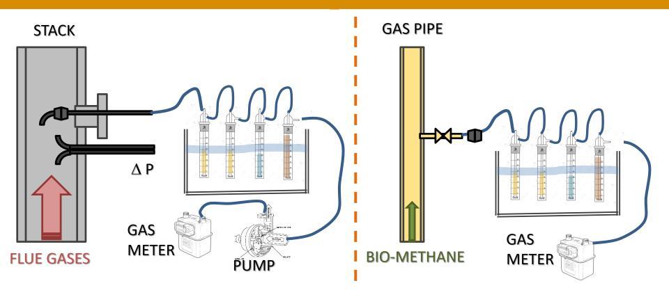
Isokinetic conditions for sampling can be neglected for bio-methane, as well as the filter
