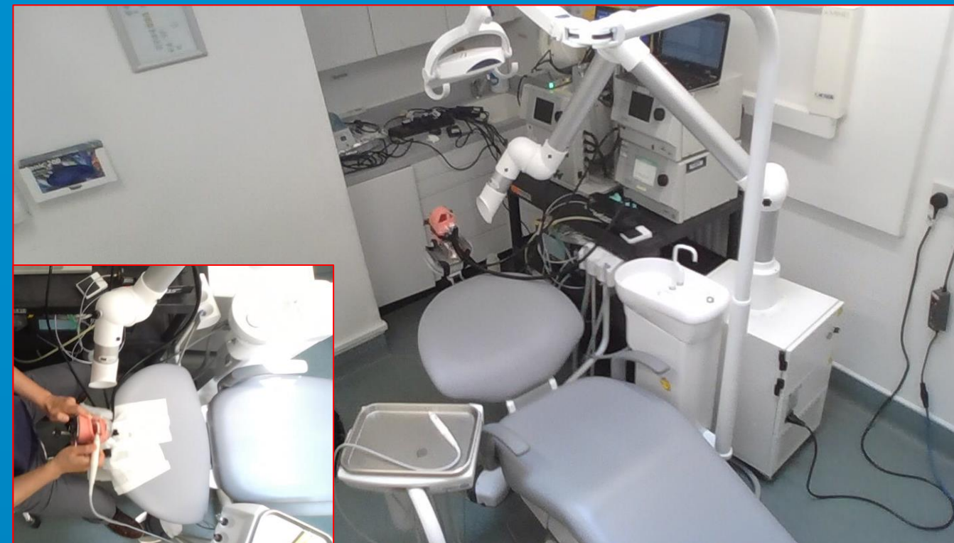
Figure 2: Equipment set up in MyDentist surgery; Inset: AGP being performed with EAFS extraction
