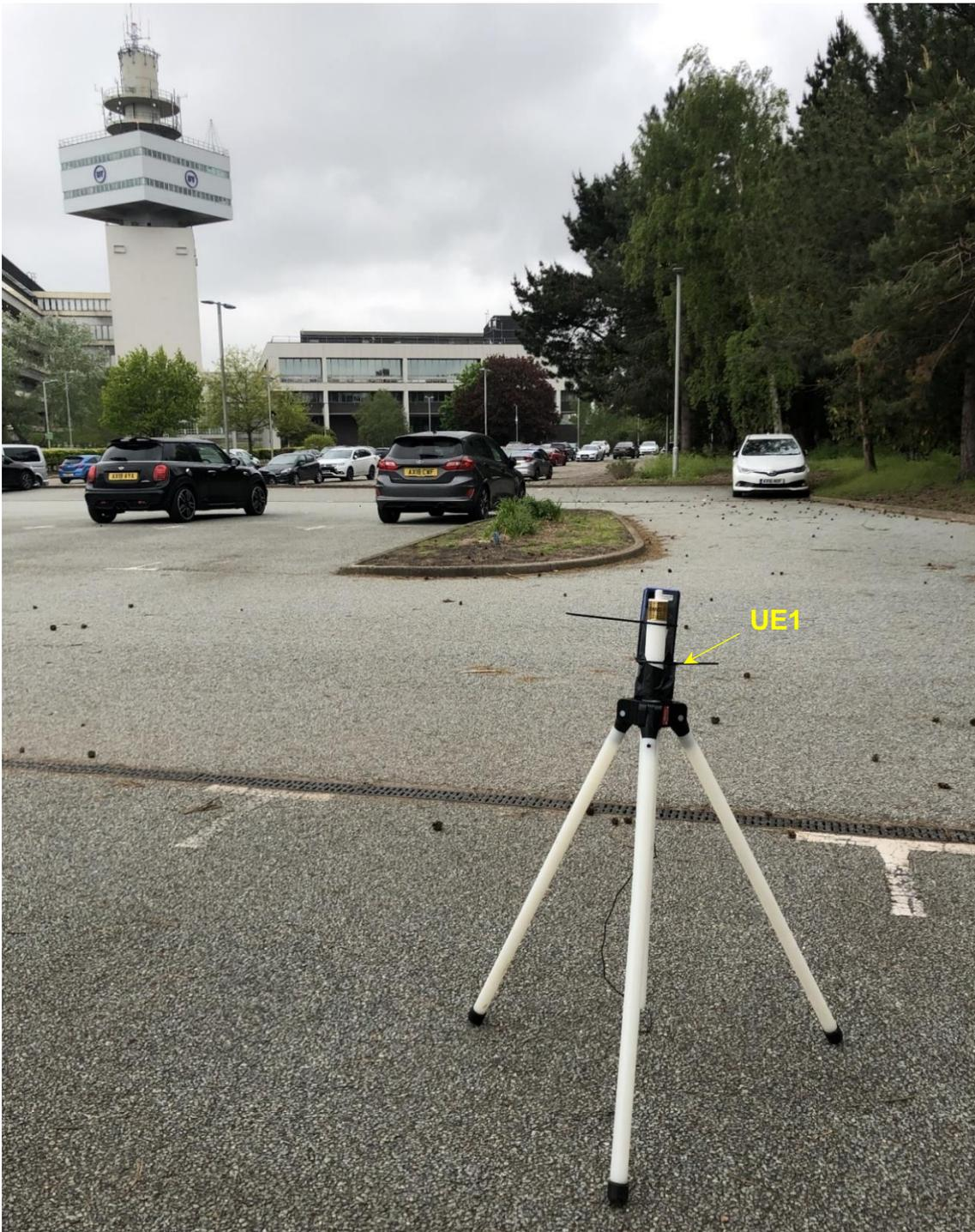
Figure 32 Measurement setup for UE1 at the UK 5G-VINNI 5G BS in an outdoor environment.
