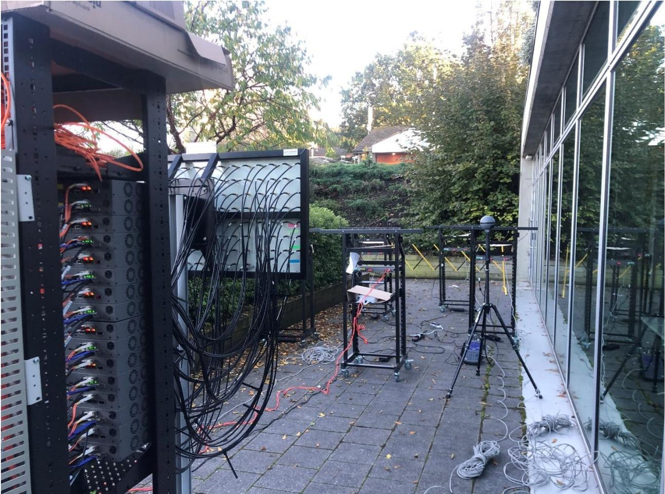
Figure 28 *Photograph of the experimental setup for the outdoor RF-EMF measurement campaign (2) for comparison between the two RF-EMF methods.*
