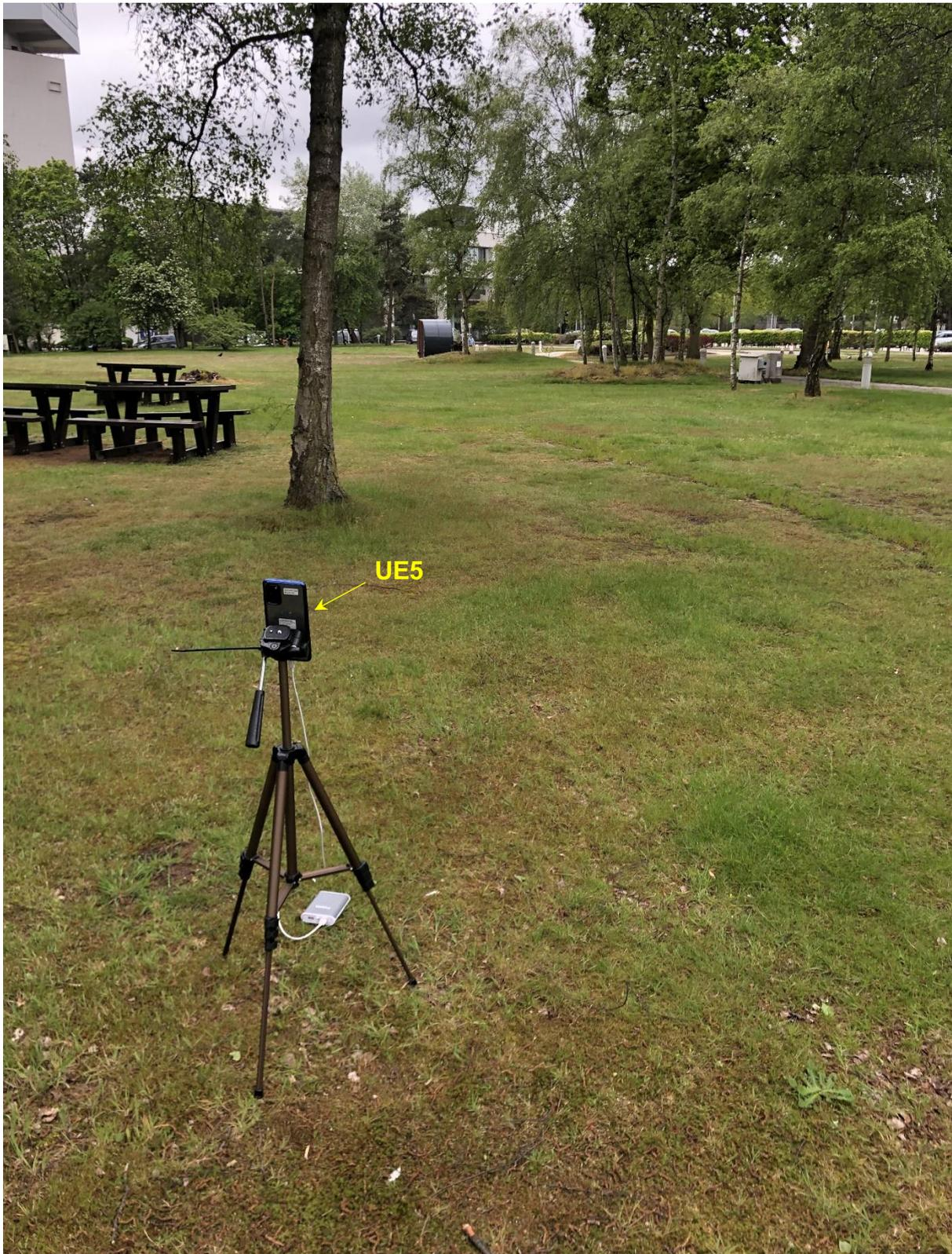
Figure 36 *Measurement setup for UE5 at the UK 5G-VINNI 5G BS in an outdoor environment.*
