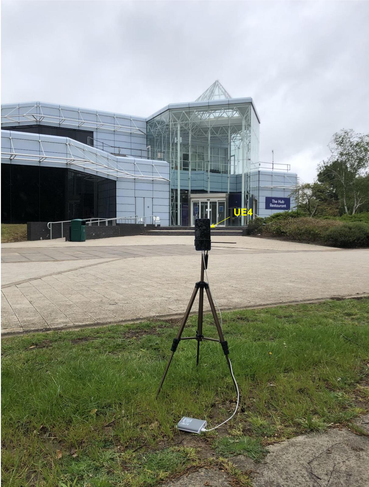
Figure 35 Measurement setup for UE4 at the UK 5G-VINNI 5G BS in an outdoor environment.
