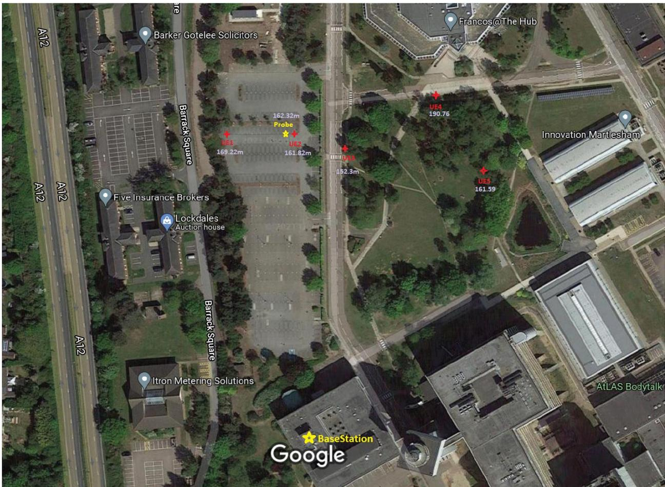
Figure 31 Measurement setup for the RF-EMF assessment of a commercial 5G BS in an outdoor environment at UK BT Adastral Park site in Ipswich. Note that the distance of each UE from the BS is marked at the UE.
