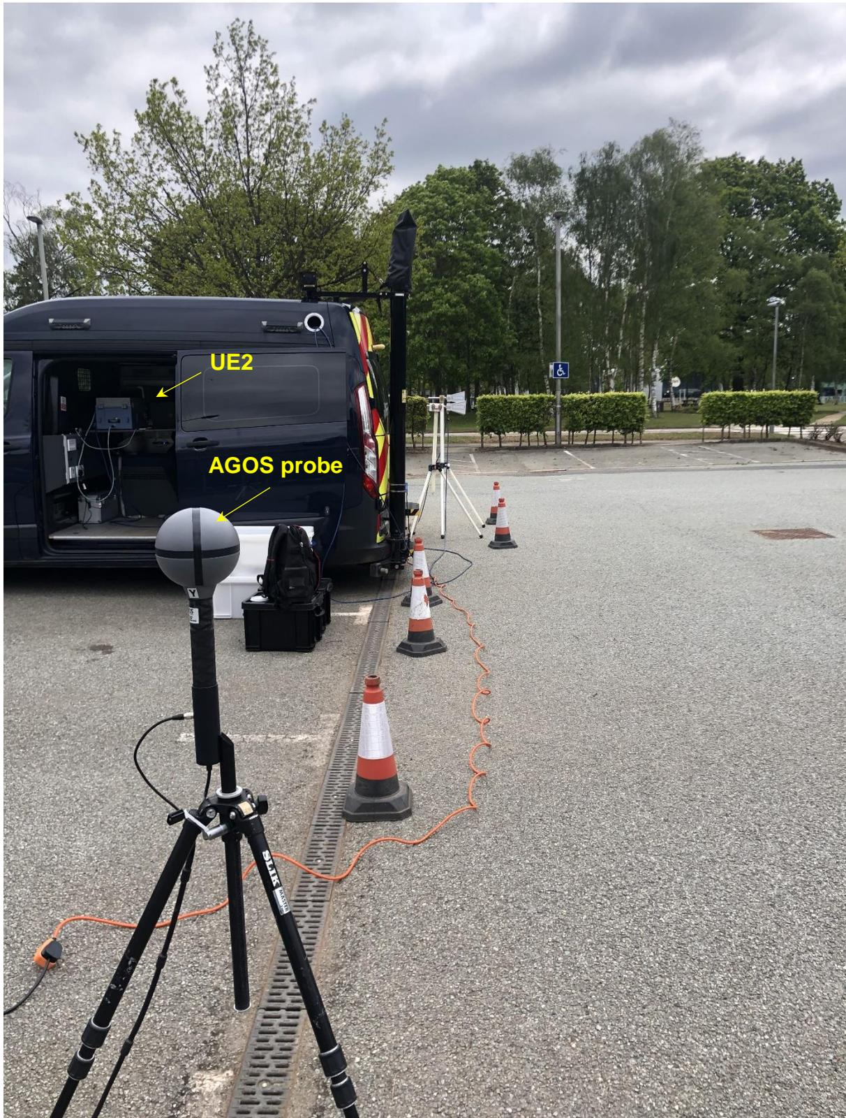
Figure 33 Measurement setup for UE2 and the Keysight RF-EMF measurement system for the assessment of the UK 5G-VINNI 5G BS in an outdoor environment.
