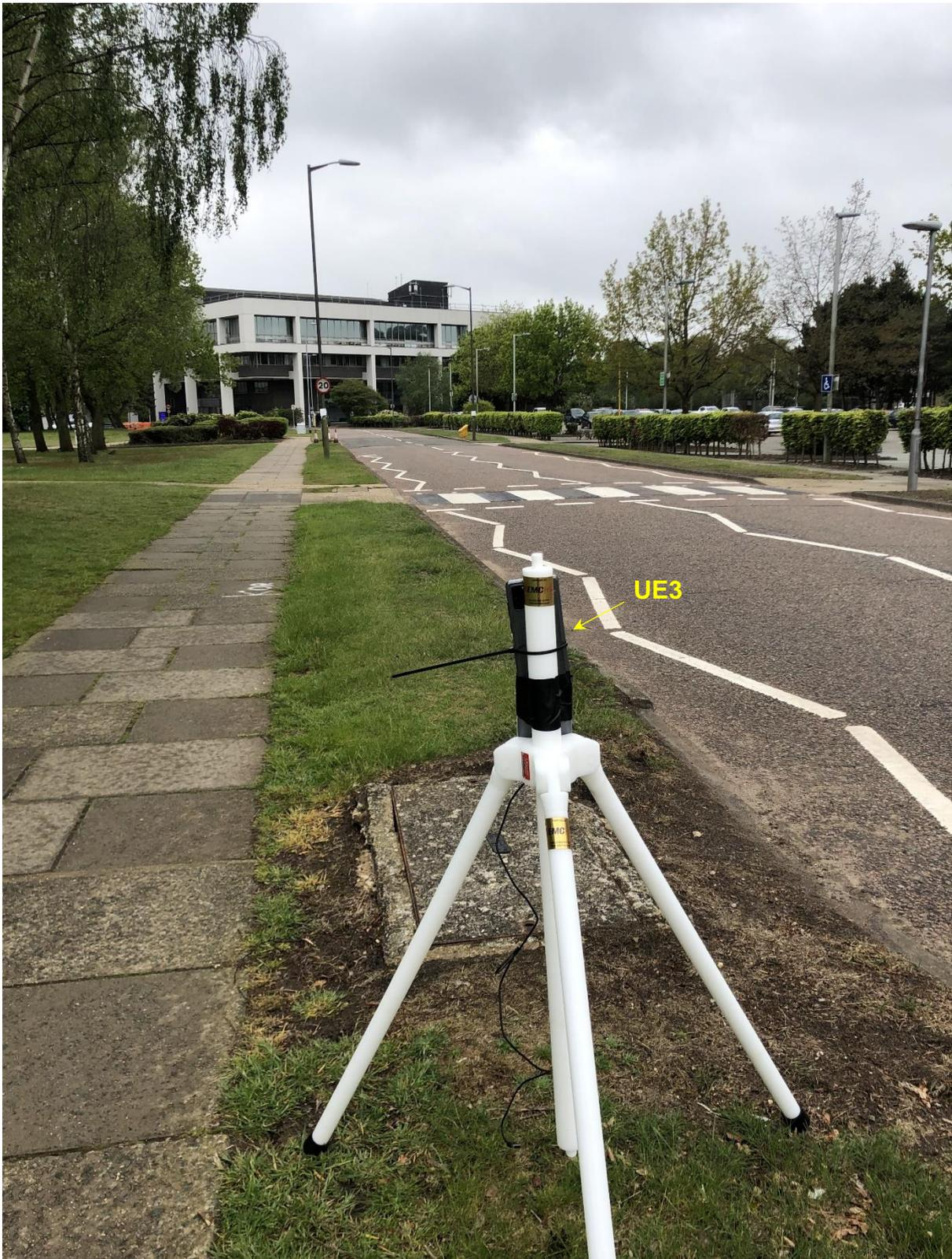
Figure 34 *Measurement setup for UE3 at the UK 5G-VINNI 5G BS in an outdoor environment.*
