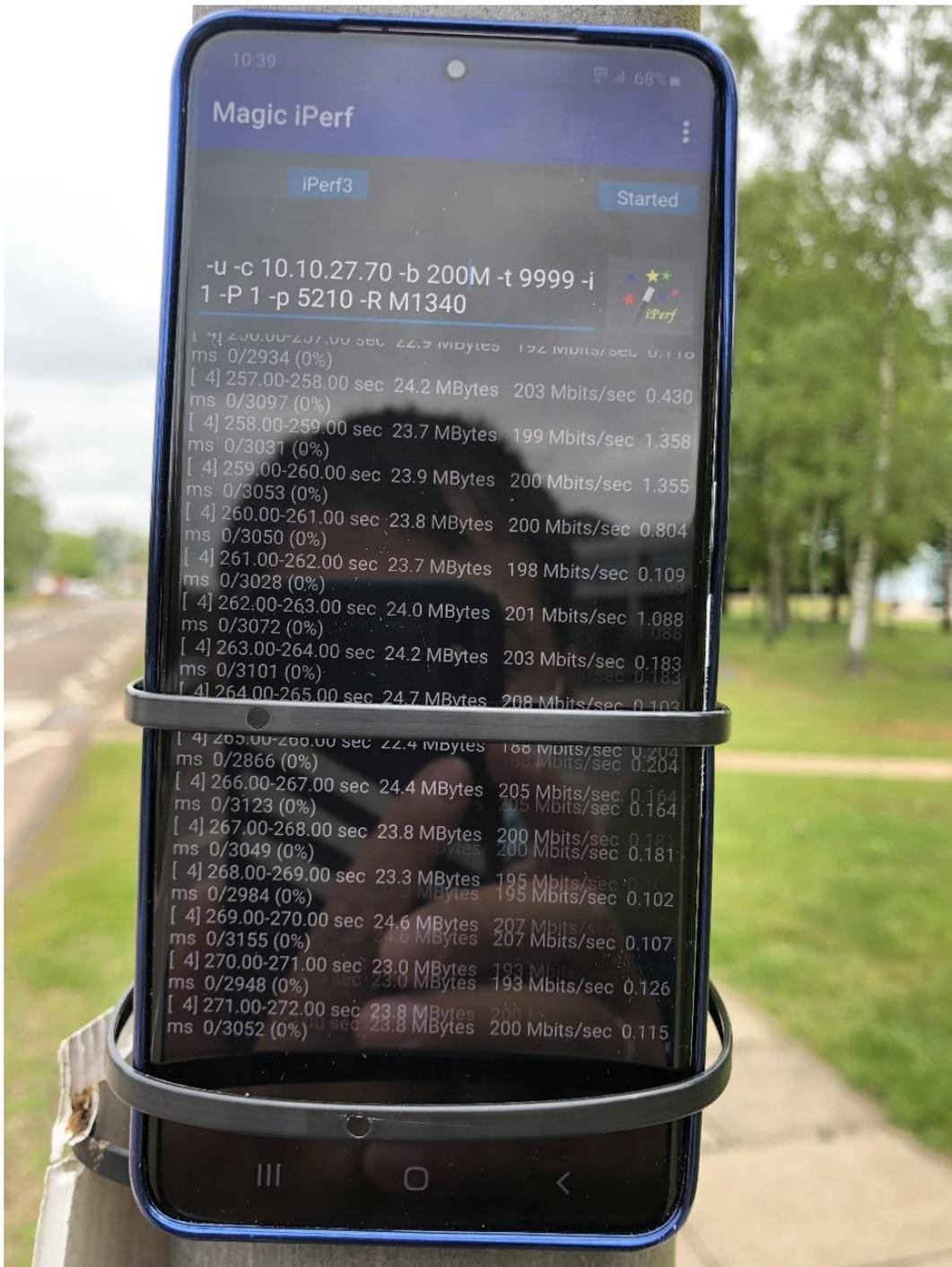
Figure 37 Measurement setup for the RF-EMF assessment of the UK BT 5G BS in an outdoor environment.
