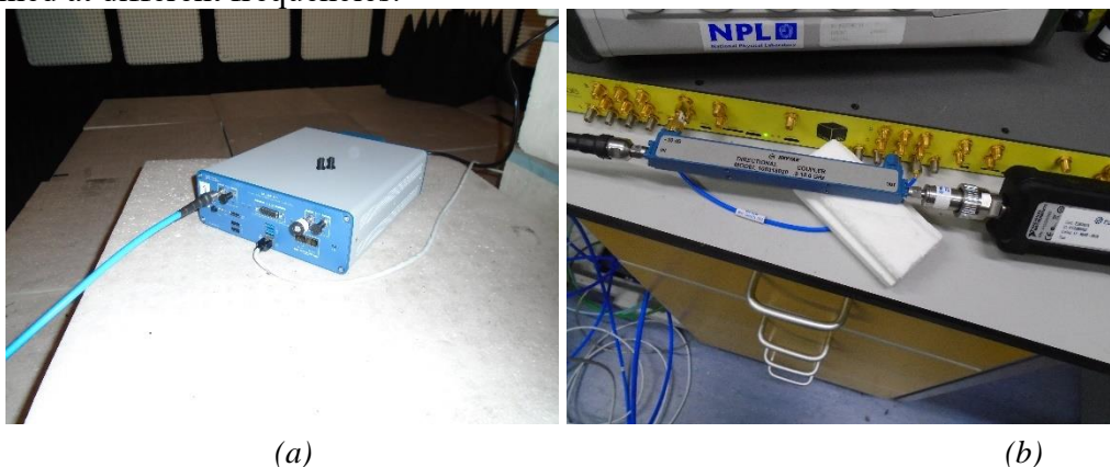
Figure 16 Photographs of the: (a) signal generator used to generate the calibration waveform; (b) directional coupler connected to the megabee and power sensor.
