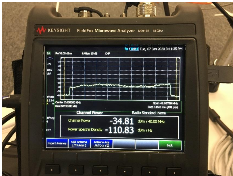
Figure 23 Channel Power measurement for 5G NR using Keysight RF-EMF measurement system.
